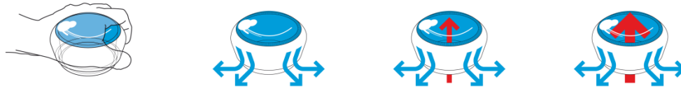
Figure 1: Schematic depiction of the thermal currents in the adjusting knob (thermal display). Variable heat generation (red arrow) and constant heat removal (blue arrows)
